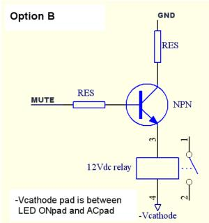
Option B shows the circuit with a relay output. The relay can have more than the one set of contacts shown on the schematic which make it possible to control either signal input or output of the amplifiers.
