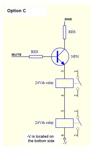
Option C shows how to implement two relays which offers the possibility of more sets of contacts. Note that the circuit now is supplied from the power amplifier supply to ensure enough voltage for the relays.
