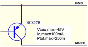
The above schematic shows the mute output circuit. The output needs no glue components if it has to control our own power amplifier modules PA1CC, PA3CC and PA6CC.
