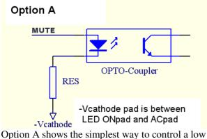
Option A shows the simplest way to control a low power enable control input of the amplifier module. The transistor output might have to be a Darlington coupling and/or have to have a series resistor.
